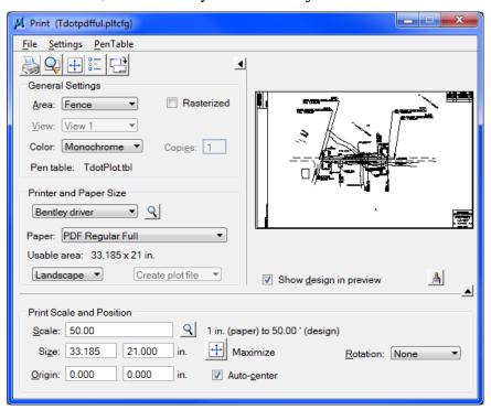
6. In the MicroStation Print dialog go to **File> Print** or click the printer icon on the dialog. The **Save Print As** dialog opens. Adjust the folder and filename as needed and click **OK** to save the PDF file.
